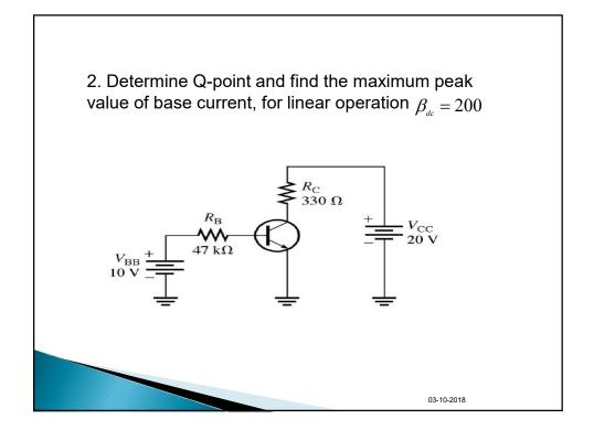
$$\begin{split} & I_B = \frac{V_{BB} - V_{BB}}{R_B} = \frac{10V - 0.7V}{47K\Omega} = 198\mu A = I_{BQ} \\ & I_C = \beta_{DC} I_B = (200)(198\mu A) = 39.6mA = I_{CQ} \\ & V_{CB} = V_{CC} - I_C R_C = 20V - 13.07 \\ & = 6.93V = V_{CBQ} \end{split}$$
