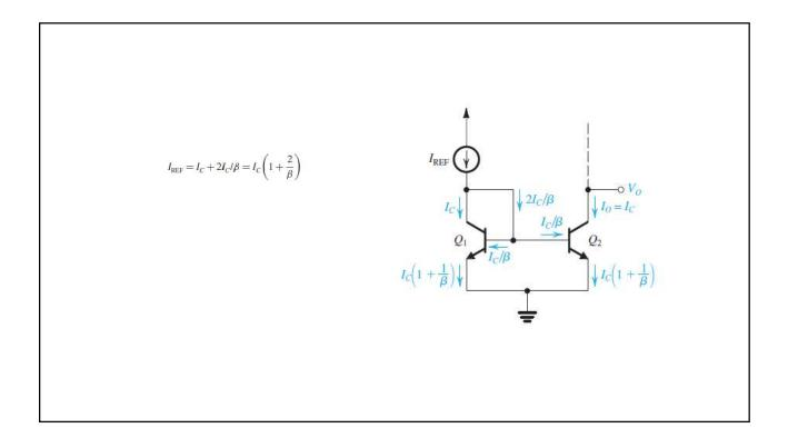
Finally, since  $I_0 = I_c$ , the current transfer ratio can be found as
