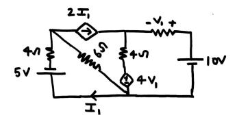
(c) Calculate V1 and current in 4 ohm resistance
